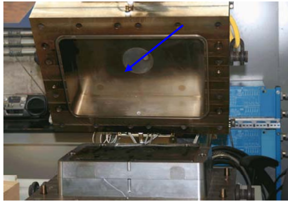
Fig. 2 Dielectric sensor location in the RTM mold.
